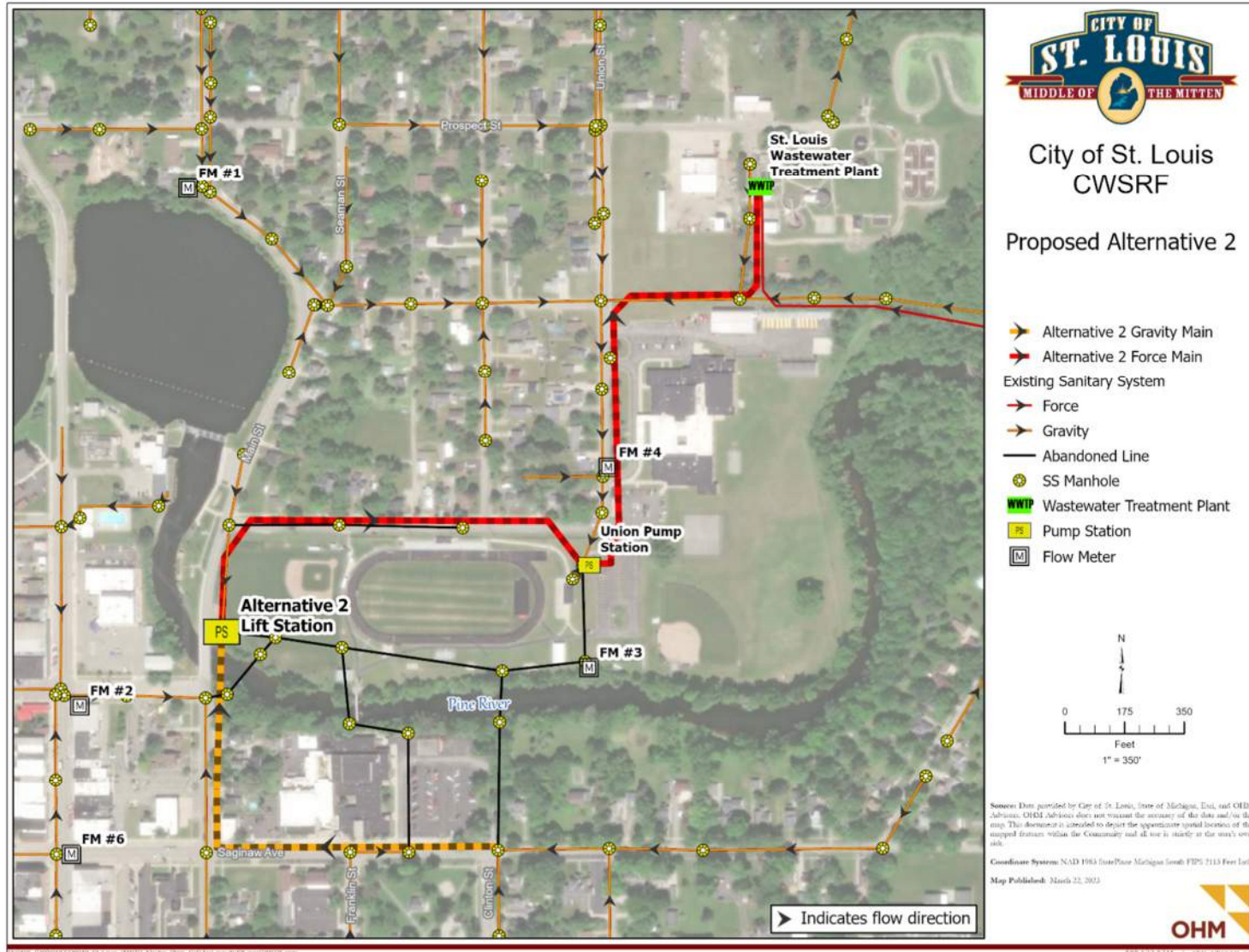
Figure 3-2: Alternative 2 Collection System Layout
