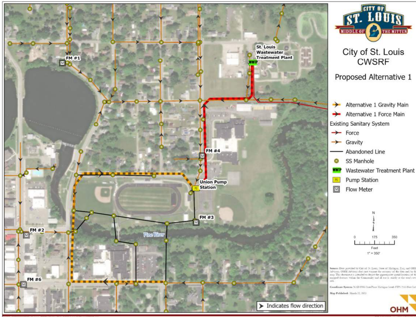
Figure 3-1: Alternative 1 Collection System Layout
